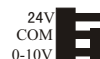
The position of shorting bar when the voltage input signal is applied
