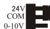
The position of shorting bar when transducer power is supplied by the instrument
